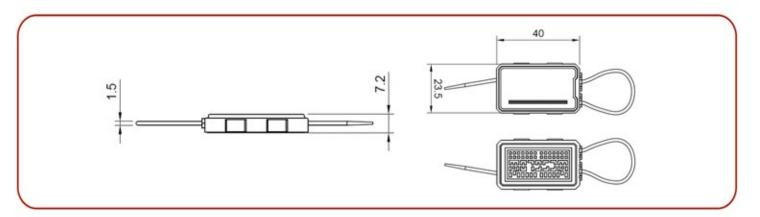
Cable grip seal has a robust lock that is covered by special designed ABS housing
