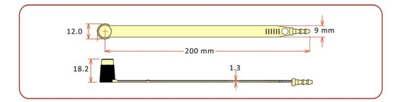
The TwinLock fix-length or fix-loop seal with double-lock design It is made of 2 kinds of plastic to resist heat & solvent attack.
