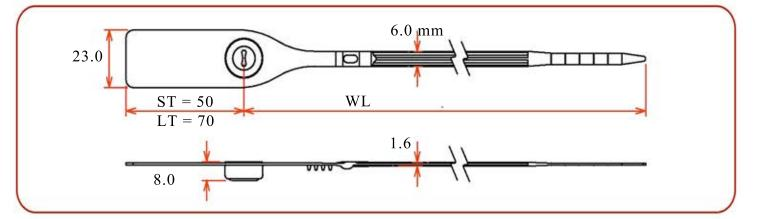
With stainless locking jaw for improved security. Used widely for securing valued cargo or when high strength is needed.
